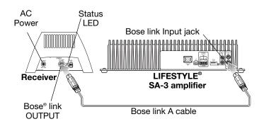
Insert the small plug on the power pack cable into the AC Power jack on the receiver and plug the pack into a wall outlet.
